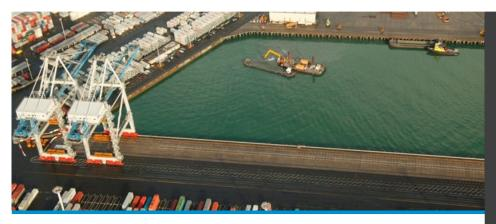
Heron Construction completed the dredging of 750,000m<sup>3</sup> of marine sediment, clays and sandstones from the Rangitoto Channel and the Fergusson Approaches and turning basin using the backhoe dredge Kimahia.
