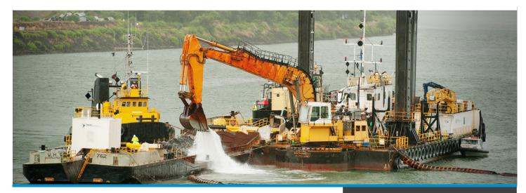
The backhoe dredge Machiavelli was used to dredge a combination of rock, stiff clays and marine sediments from the Hunter River for departure channel for the newly completed Newcastle Coal Infrastructure Group's Kooragang Berth K8 and K9.
